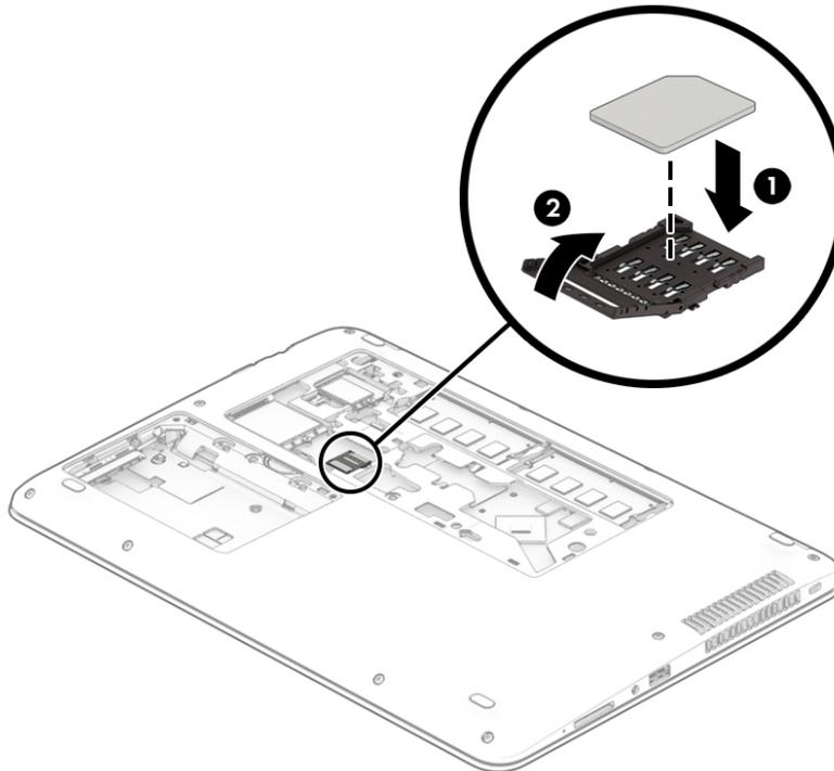
To remove a SIM card, rotate the SIM connector hinge upward, and then remove the SIM card from the connector.
