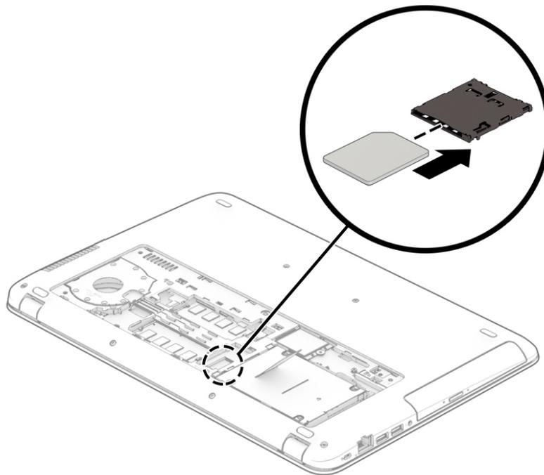
To remove a SIM card, press in on the SIM card, and then remove it from the slot.
