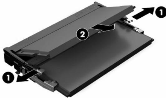
4. Slide the new memory module into the slot (1) at approximately a 30° angle, then press the memory module down (2) so that the latches lock it in place.
